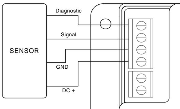
Sensors can be NPN or PNP output. Sensor signal line must be on when a unit is blocking the sensor. Consult the sensor manufacturers' documentation for details.
