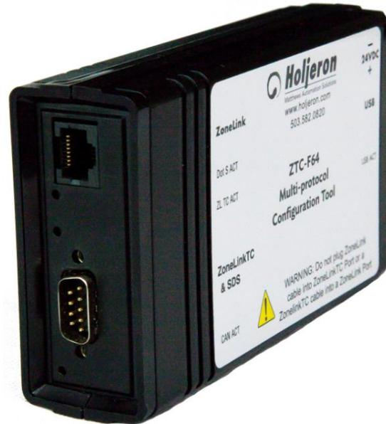
**Please Note: If you intend to use the ZTC-F64 tool with both ZoneLink®.S and ZoneLink® TC installations, care must be taken to connect the device to the appropriate network.**
