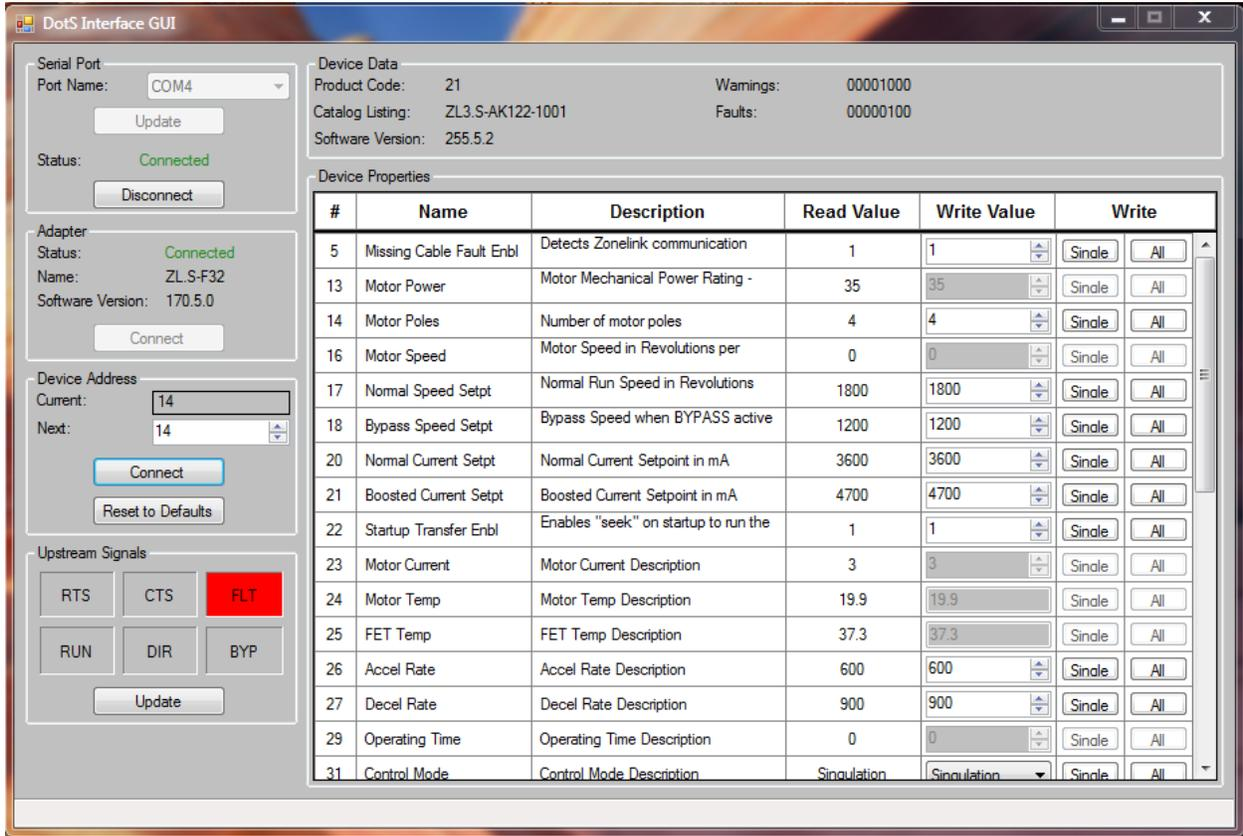
In order to change a setting, modify the value in the “Write Value” column. Hit the “Single” button in the “Write” column to write only to the unit specified in the “Device Address” box in the left pane, or hit “All” to write that value to all of the units on the bus.
